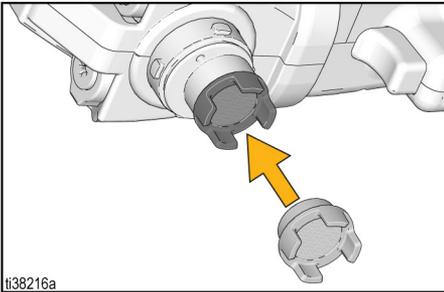
5. Install the cup assembly onto the sprayer as follows:
