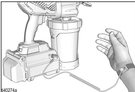
3. The included heel grounding strap ensures a positive ground to the floor. To attach the heel grounding strap, follow these steps:
