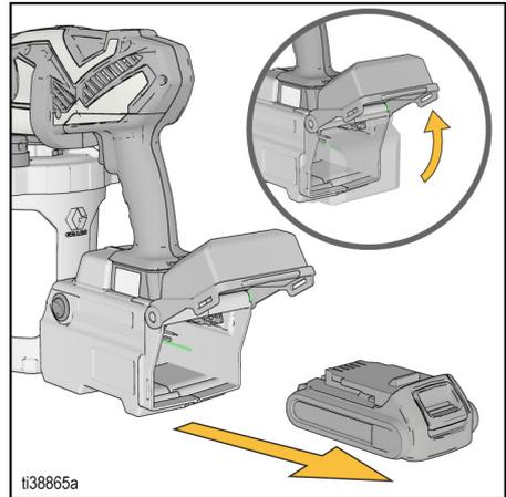
3. Install fully charged Battery into the sprayer.
