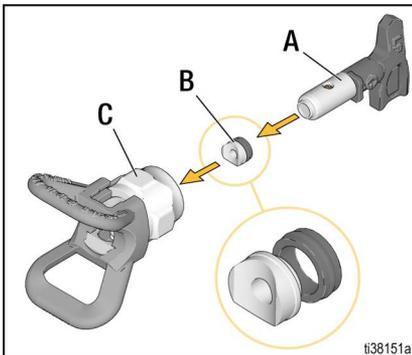
3. Insert Spray Tip into Spray Tip Guard. Verify Spray Tip is forward in the SPRAY position.
