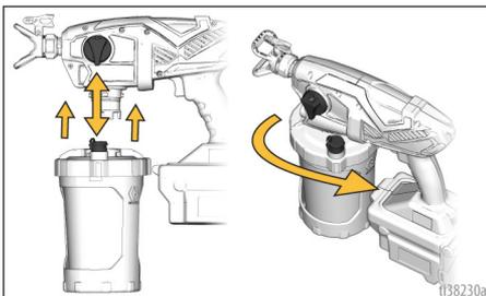
6. Install Battery into the sprayer.
