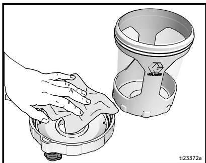
20. Wipe disinfectant off the outside of the sprayer using a soft cloth moistened with water.
