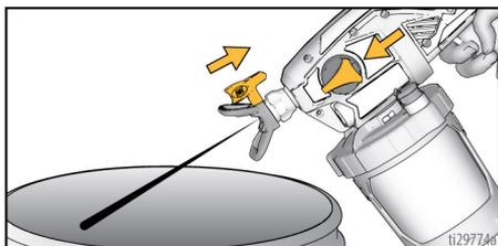
5. Turn Prime Knob downward to PRIME position. Rotate Spray Tip back to SPRAY position. Turn Prime Knob forward to SPRAY position, and resume spraying.
