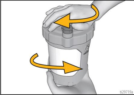
4. Verify Pump Filter is installed and clean.
