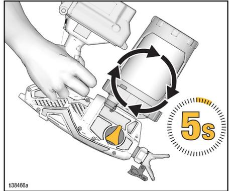
9. Rotate Spray Tip 180 degrees to UNCLOG position. Turn Prime Knob forward to SPRAY position.
