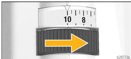
4. Point sprayer into waste bucket, turn Prime Knob forward to SPRAY position. Pull Trigger for 5 seconds to clear clog.
