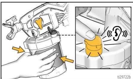
**NOTE:** If FlexLiner is not squeezed while VacuValve Cap is open, air will quickly pull into the FlexLiner. If any air bubbles are visible in the cup, repeat steps E-G.
