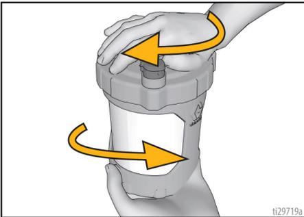
5. Install the cup assembly onto the sprayer as follows:
