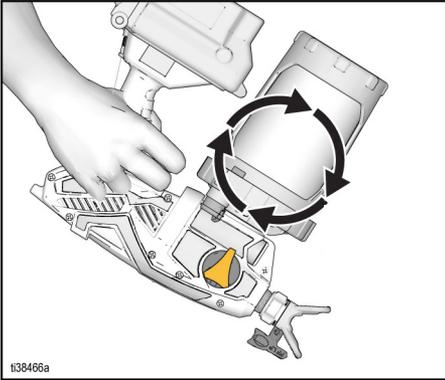
12. Verify Spray Tip is forward in the SPRAY position. Turn Prime Knob forward to SPRAY position.
