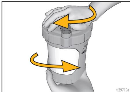
9. Install the cup onto the sprayer.
